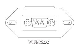
This RS232 port is used to connect the wifi datalogger
