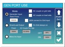
Generator input rated power: allowed Max. power from diesel generator.
