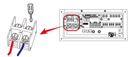
For 7.6KW/8KW model, battery connector screw size: M10
