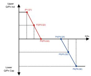
Pic 8.26 Reactive Power Regulation Curve in Q(P) Mode
