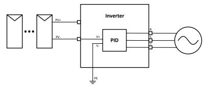
The Anti-PID module repairs the PID effect of the PV module at night. The PID module always runs when connected to AC.
