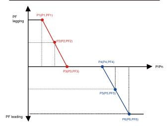
Pic 8.28 Power factor Regulation Curve in PF(P) Mode
