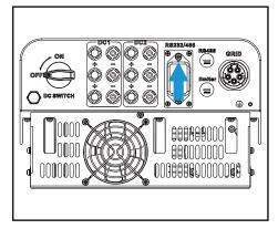
Pic 5.13 datalogger installation diagram
